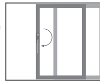
Handle pointing vertical down OPEN
